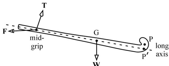
**Figure 1:** Free-body diagram of a field hockey stick, including the locations of all points used in the model.
